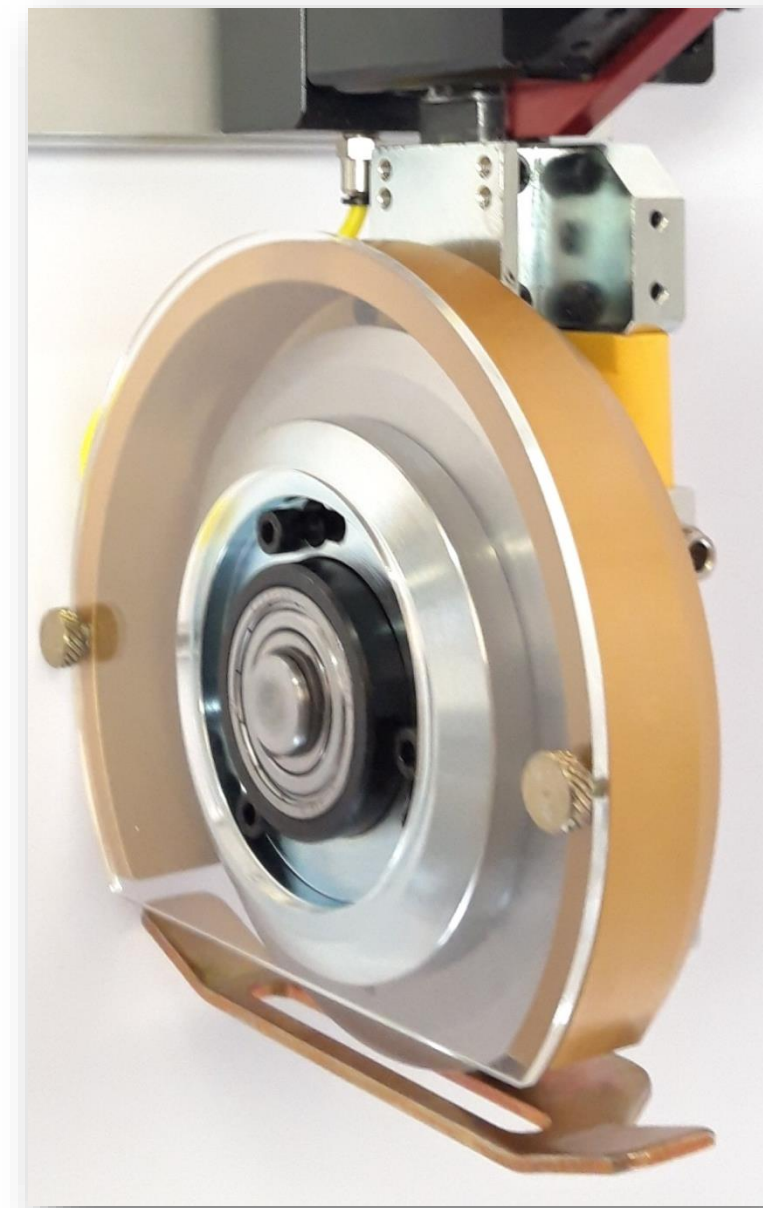
PLEXIGLASS SIDE COVER FOR BLADE
